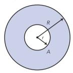
The area of an annulus can be found by subtracting the area of the inner circle from the area of the outer circle.
